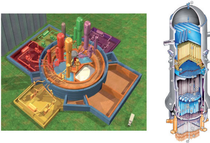
Fig. 8. – GenIII reactors based on Active Safety Systems. Left: EPR; right: ABWR.
