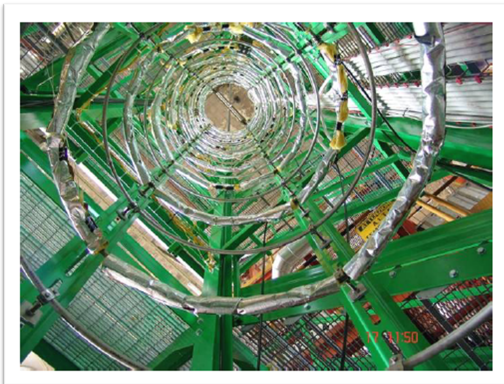
Fig.3-Pictures of Helical Coil Steam Generator test section
