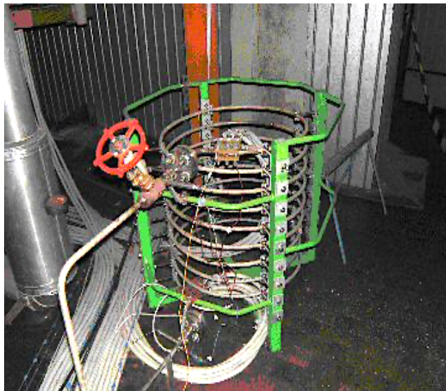
Fig.1-SIET forced flow experiences supply section schematic (a), supply section pre-heater (b)
