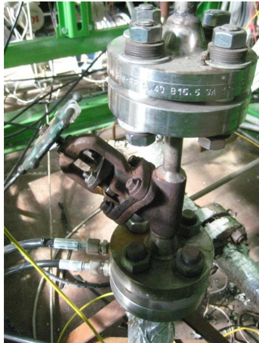
Calibrated orifice and channel inlet valve (V1 and V2 in Fig.2b).
