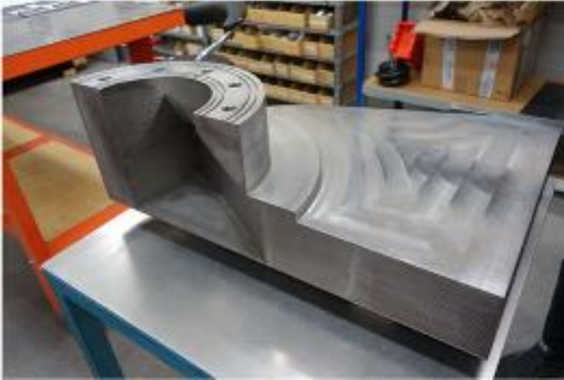
Compact Steam Generator mock-ups to setup the manufacturing process
