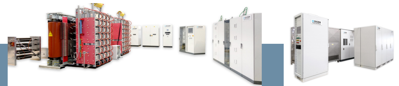
Ion Source and Extraction Power Supplies for ITER. A turn key integrated system capable to generate voltage up to 1000 kV, Energy up to 17 MW and 3600 s of pulse length
